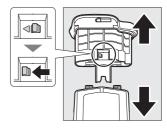
**AA batteries**: Remove the batteries as shown. Be careful not to drop the batteries when removing them from the holder.
