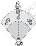
This is convenient when you need a large flash output. All the slave units will fire at the same output and be controlled to obtain a standard exposure.
