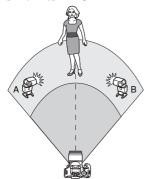
Divide the slave units into groups A and B and change the flash ratio to obtain the desired lighting effect.
