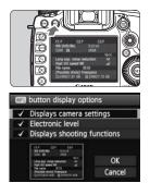
When you press the **<INFO.**> button while the camera is ready to shoot, you can display [**Displays camera settings**], [**Electronic level**] (p.60), and [**Displays shooting functions**] (p.343).
