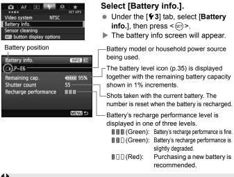
The use of a genuine Canon Battery Pack LP-E6/LP-E6N is recommended. If you use any battery other than the Battery Pack LP-E6/LP-E6N, the camera's full performance may not be attained or malfunction may result.
