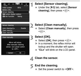
If you use a battery, make sure it is fully charged. If the battery grip with size-AA/LR6 batteries is attached, manual sensor cleaning will not be possible.
