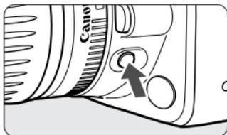
Press the depth-of-field preview button to stop down to the current aperture setting. The diaphragm in the lens will be set to the current aperture so you can check the depth of field (range of acceptable focus) through the viewfinder.
