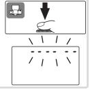
4 Holding the camera so that light falls on the low-pass filter, examine the filter for dust or lint. If there are foreign objects on the filter, the filter requires cleaning. See the following section.
