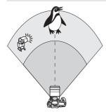
This shows the most basic setup for fully-automatic wireless flash with one Speedlite.
