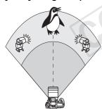
Convenient when you need a large flash output. All the slave Speedlites will fire at the same output and controlled to obtain a standard exposure.
