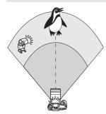
This shows fully-automatic wireless flash shooting with one external Speedlite and the built-in flash.
