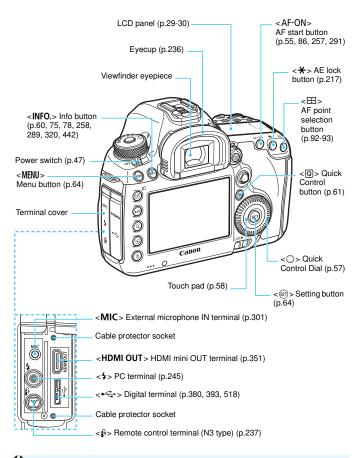
When connecting the interface cable to a digital terminal, you must use the provided cable protector (p.36).
