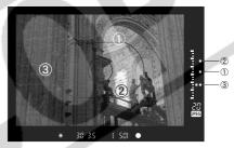
While referring to the exposure level indicator's three spot metering marks, you can set the exposure compensation to obtain the desired result.
